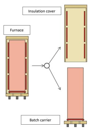
At first sight, removing the complete furnace out of the pressure vessel seems to be more laborious than simply taking off the process product. Nevertheless, our design has various decisive advantages:
