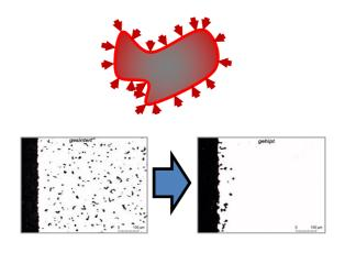
Usually, Argon is used as pressure transmitting medium at material-specific sinter temperatures, i.e. approx. 0.7 \* Ts.
