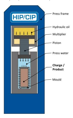
At first, the material to be compressed is put into the recipient filled with press medium. In the next step, a piston plunges into the recipient from above. The hydraulically driven piston applies big force to the press liquid, thus creating the desired pressure inside the recipient.
